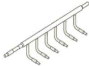
Header Liquid Pipe
